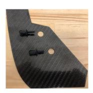
2. Under the front wheel arch at the rear at the car sill end, push the centre of the black 2 plastic clips in, to then allow their removal. Then fit the supplied front spat and reinsert the 2 clips into the holes of the c/fibre and into the arch liner and sill end. If needed you can instead always drill the two holes out carefully to 10mm and then drill two new 5mm holes (as shown below)and fit the supplied 5mm diameter powder coated rivets
