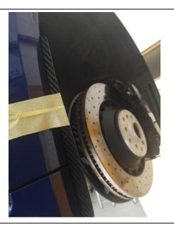
Handbrake on Loosen the wheel bolts 1<sup>st</sup> with the correct tools as per Audi handbook
