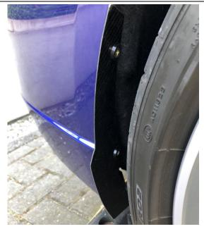
4. Rears unscrew the two screws from the arch lines, then fit the new spats with the long non tapered nylon spacer at the bottom and supplied c/cunk alloy black washer and gold 5x50mm wood screw. In the top hole use the nylon spacer with the 45 degree chamfer and again wood screw and c/sunk alloy washer, make sure you turn the spacer so the chamfer angle helps pull the spat to the shape of the liner.
