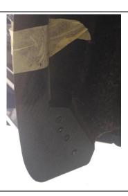
3. Now very carefully apply some superglue behind the upper part of the front carbon spat to bond it to the plastic arch lip liner. Make sure the glue does not run onto the c/fibre and spray some activator on whilst it is held or masking taped inplace. For best effect we use a black methacrylate fast drying adhesive top and 3" down and a dab of super glue in the middle between the other adhesive. Allow to set fully before removing tape.
